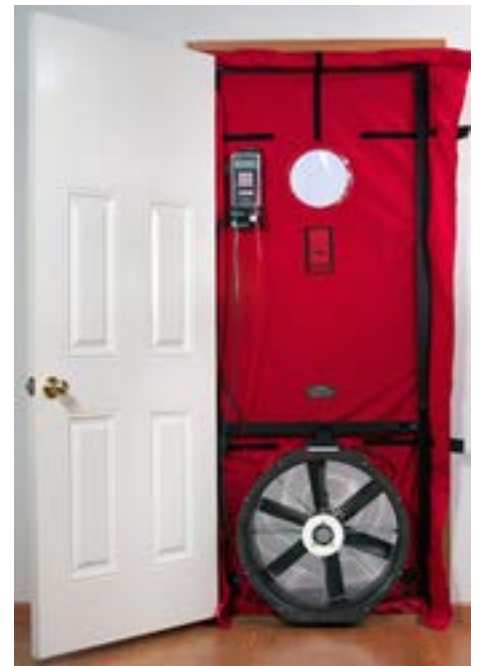
Example of blower door test.
