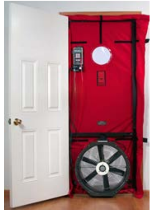
Example of blower door test.
